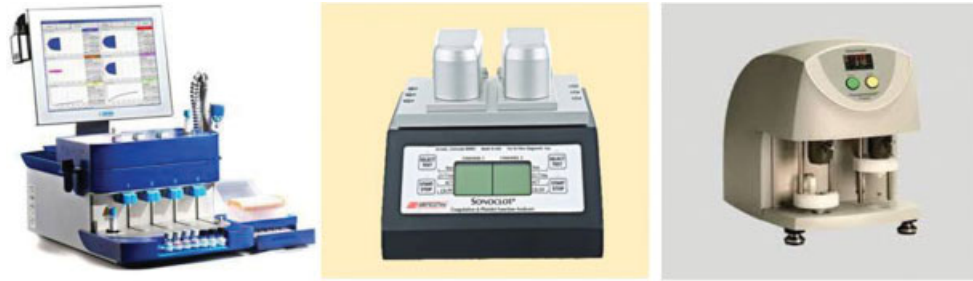
Fig. 1 (A) Platelet aggregometry using rotational thromboelastometry; (B) platelet aggregometry using Sonoclot; (C) platelet aggregometry using thromboelastography.
